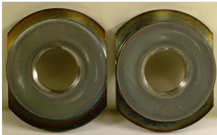
Fig. 2 Photograph of the crevice surfaces after test #1, 1.5 % HCl at 80 °C
