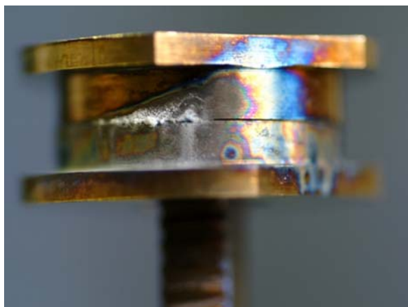
Fig. 6 Photograph of the crevice cell after test #3, 25 % NaCl at 100 \text{ }^\circ\text{C}
